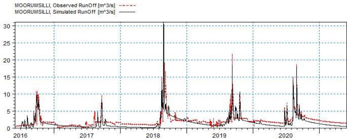
Figure 5.16 Comparison between observed and simulated discharge for Murumsilli during validation.
