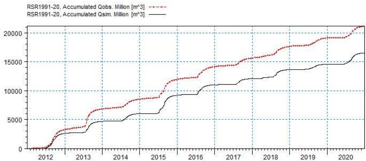
Figure 5.23 Double Mass Curve for Ravishankar Sagar reservoir during validation period.
