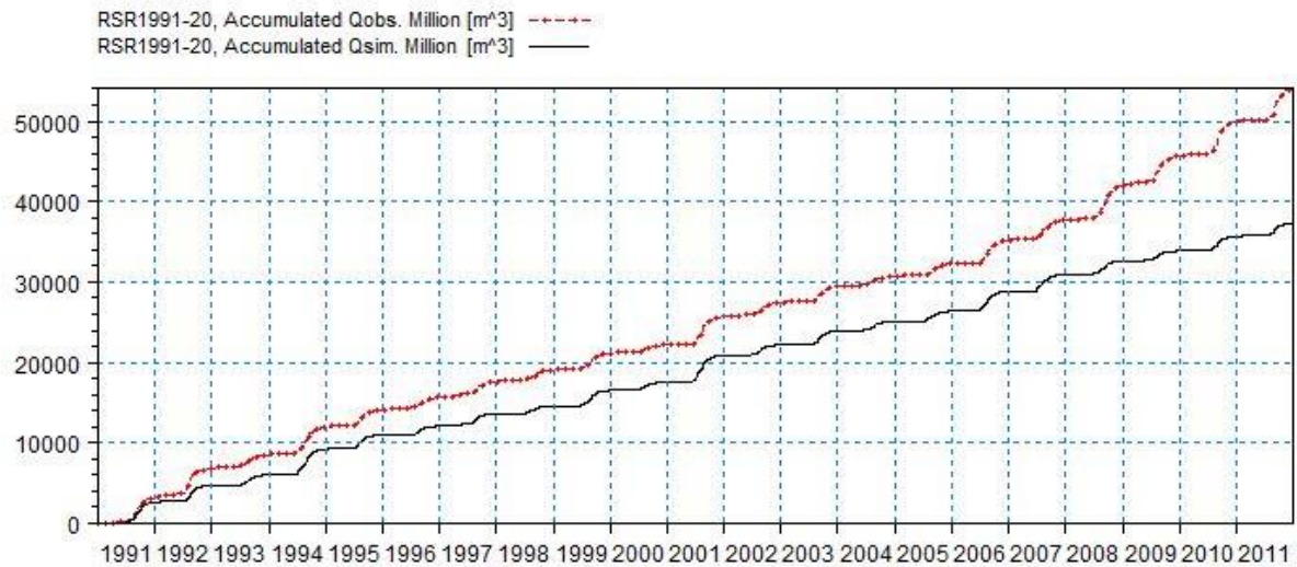
Figure 5.20 Double Mass Curve for Ravishankar Sagar catchment during calibration period.
